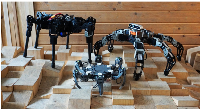
FIGURE 8. HAntR (left), PhantomX AX (right), and small hexapod walking robot with Dynamixel XL-320 servomotors (middle) on the rough terrain testbed.
