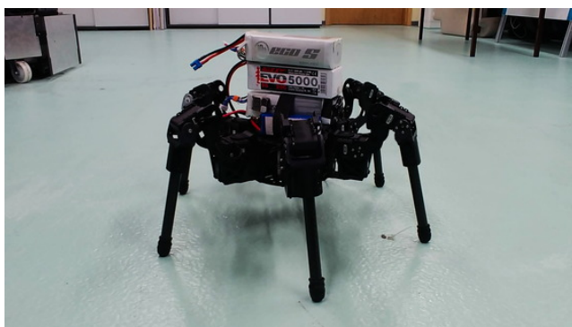
(a) Without additional payload. (b) Additional payload. (c) Robot carrying 2460 g of additional payload. FIGURE 12. Evolution of the mean temperature of the robot servomotors during the endurance experiment and the robot carrying the additional payload.
