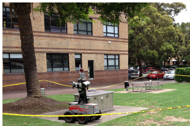
Fig. 7 The robot moving through the environment and using its onboard Velodyne laser scanner to collect the 3D point-cloud dataset (Patten et al. 2015)
