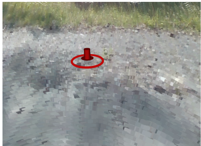
Fig. 15 The area (red circle) around a point of interest (red marker) signifying the cells used to compute the histogram terrain descriptor, projected on the elevation map with localized color measurements.
