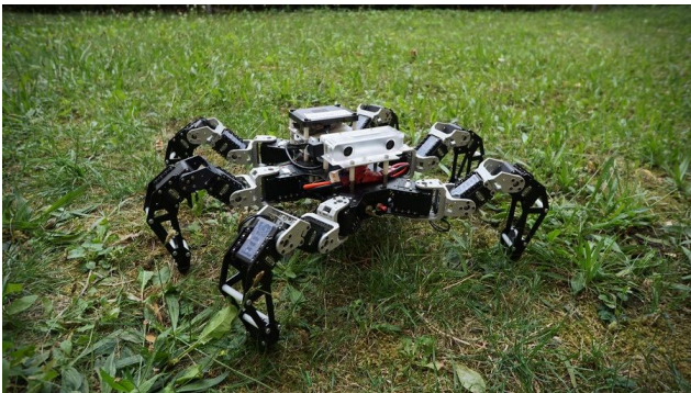
Figure 1. Utilized hexapod walking robot with mounted wide-angle lens stereo camera.
