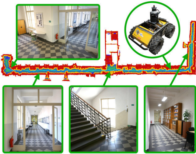
Fig. 6. Visualization of the dense map created during the experimental deployment as a union of local maps used for precise navigation. The topological map is marked by cyan color. Parts of the environment and the wheeled robot are shown in the included photos, where an arrow from the robot's photo points to the robot's location.
