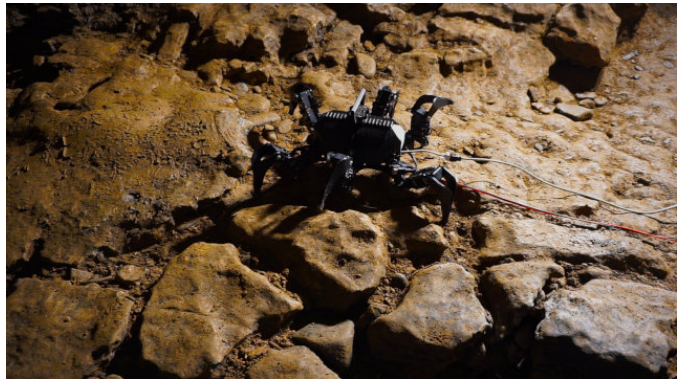
Fig. 1. Six-legged walking platform SCARAB deployed in an adverse underground environment, where the robot struggles with mud changing the weight of the legs.
