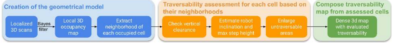
Figure 6: A schema of the local elevation map creation and traversability assessment.
