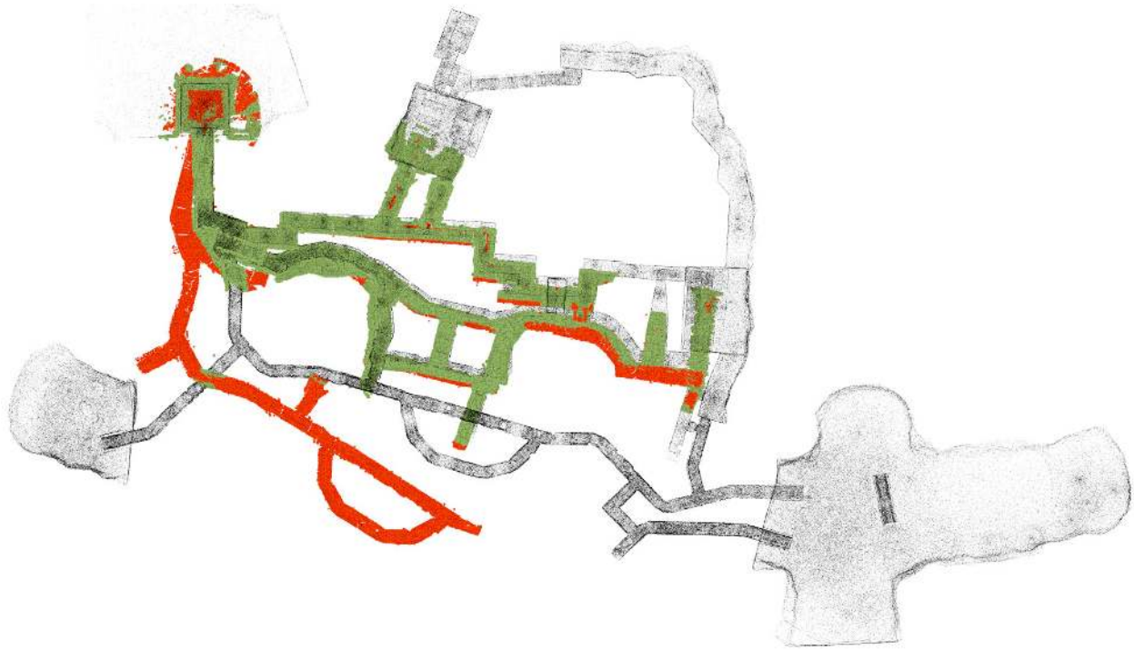
Figure 26: Map coverage and error visualized for joined local maps received from all the robots deployed in the Post-event testing in the Final circuit environment. Ground truth is black, inlier points are colored green, and outlier points are red.
