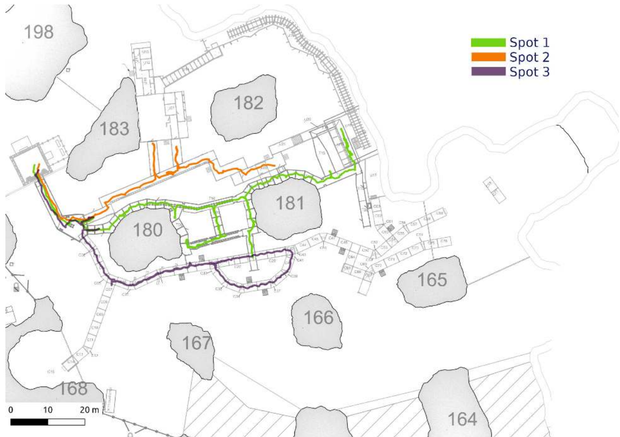
Figure 24: Paths taken by the quadruped robots in the fully autonomous mission of the Post-event testing scenario. The mapping error is captured in Fig. 26.
