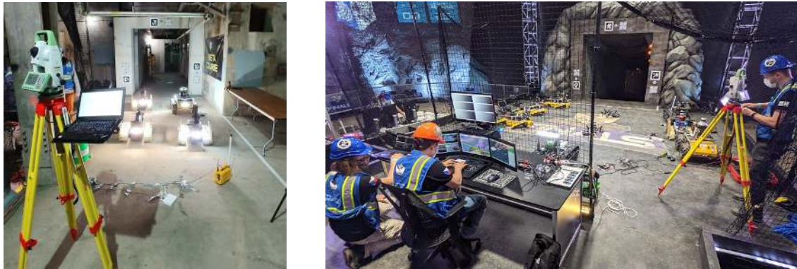
Figure 3: The robots line up in front of the entry gate to the mission area for (left) the Urban circuit and (right) the Final circuit at the beginning of the run. The coordinate frame of the robot is initialized using the Leica TS-16 total station with a laptop computer mount and the retroreflective markers attached to the robot and entry gate.
