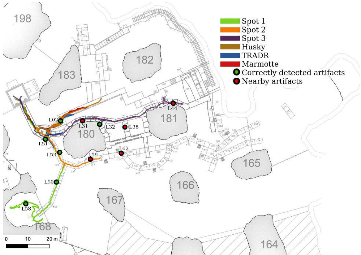
Figure 21: Artifacts detected by the ground robots and paths showing where the UGVs traversed through the Final circuit of the Systems track. The mapping error is captured in Fig. 23. The small red disks denote nearby not correctly detected artifacts.
