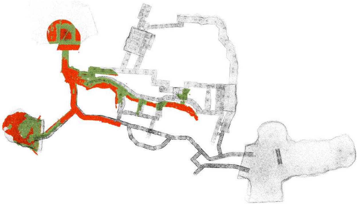
Figure 23: Map coverage and outliers visualized for joined local maps received from all the robots deployed in the Final circuit. Ground truth is black, inlier points are colored green, and outlier points are red.
