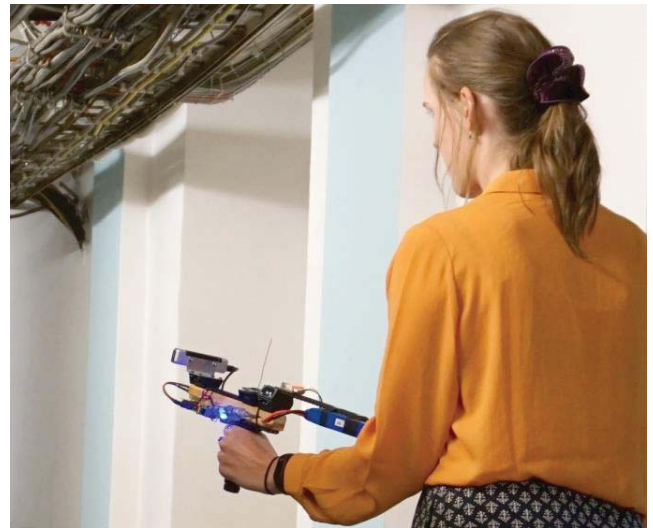
Figure 1. The prototype of the proposed handheld localization broadcaster device (light version).
