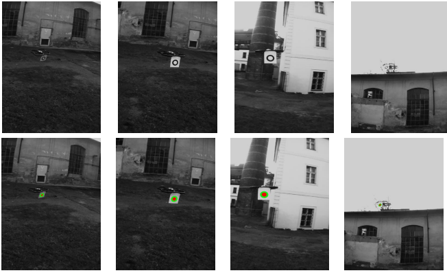
Fig. 3. Detection of the pattern attached to a flying MAV.
