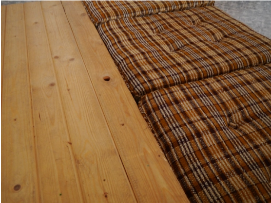
Fig. 5. Indoor testing environment – wood and pillows. According to \mathcal{T}_C classes, the surfaces were assigned as follows: \text{On} – wood, \text{Off}_{\text{right}} – wood–pillows, \text{Off}_{\text{left}} – pillows–wood, \text{Off} – pillows.
