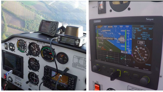
Fig. 14. Aircraft pilot panel with integrated Safely system – build-in EFIS Integra, Zaon PCAS with GPS on the flight panel and rest of the system integrated under the panel
