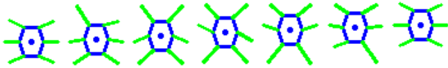
Fig. 6. Discretization of the transition between two configurations. One leg swings at a time according to pentapod gait.
