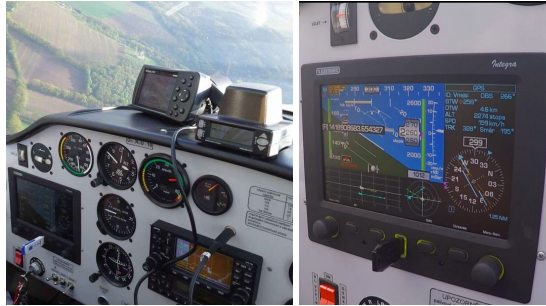
Fig. 20: Aircraft pilot panel with the integrated Safefly system – build-in EFIS Integra, Zacon PCAS with GPS on the flight panel and rest of the system integrated under the panel
