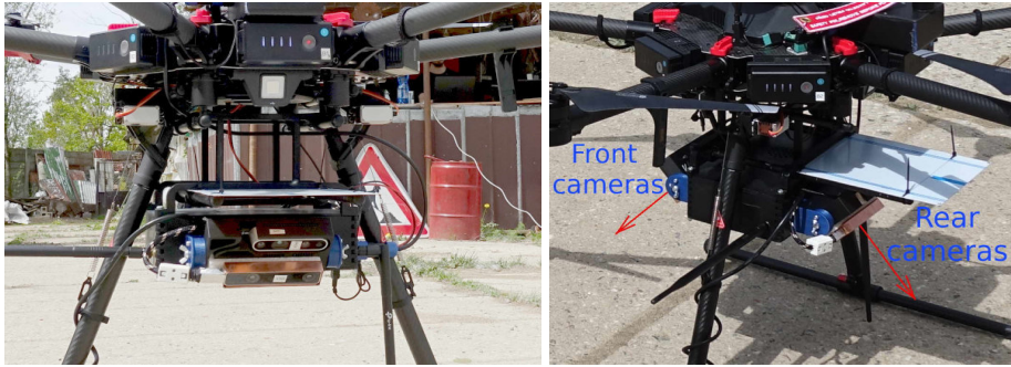
Fig. 5. The sensory equipment used during the experiments attached to the UAV; the first pair of the Intel RealSense cameras is pointed to the front. The second pair is pointed to the rear side.
