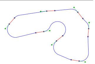
FIGURE 1. An example of the DTSP-CM instance with straight collecting maneuvers in a cargo airdrop mission. Target locations are depicted as small green disks, maneuvers are the red straight line segments, and particular trajectories for a reliable cargo drop-off are in green. The blue curves stand for the Dubins maneuvers which connect the determined collecting maneuvers into the closed tour.
