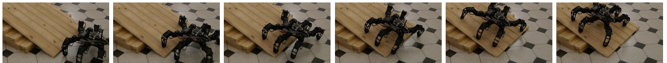
Fig. 7. Hexapod traversing an inclined plane (20° slope).
