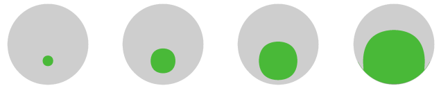
Fig. 3. Visualization of the utility introduction in the frontwave propagation for selecting the next goal. The gray circle represents a reachable area. The absence of obstacles allows the emerging frontwave to freely evolve from the robot position (slightly displaced downward relatively to the center of the circle) till the borders of the gray area, which in this particular case represents the boundary between explored and unexplored regions.
