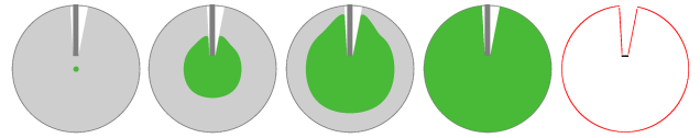
Fig. 2. A wavefront evolution in determination of the goal candidates. The light gray circular area corresponds to an omnidirectional sensor data (laser range scanner), whilst the dark gray rectangle in the top of the scene is an obstacle, which is completely drawn to improve clarity of the figure as only its edges can be sensed by the laser scanner. The green wavefront evolves from the robot position, covering all the discovered area till it reaches a static situation. The rightmost figure represents the final border reachable by the robot (depicted in red).
