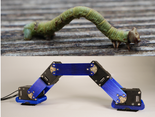
Figure 1: The considered robot resembles an inchworm with designed anisotropic friction pads with flexible scales for anchoring.
