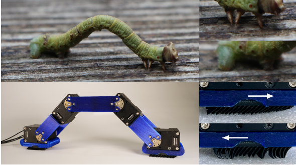
Figure 1: The designed robot resembles an inchworm with anisotropic friction pads formed by flexible scales for anchoring instead of the limbs found in its biological original.
