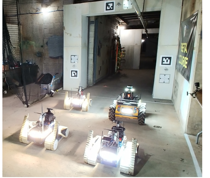
Fig. 3 The initialization process of the coordinate frames of the robots using a gate with various types of markers before the mission of the DARPA SubT Challenge.
