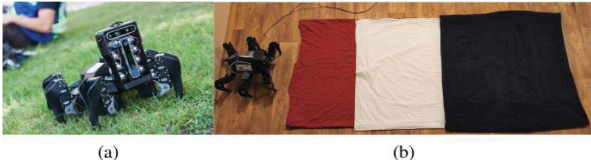
Figure 2. (a) The utilized hexapod walking robot [18] with the Intel RealSense T265 and D435 cameras, providing localization and visual perception with depth information, respectively. (b) Illustration of the robotic setup.
