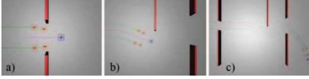
Fig. 6. Ability of deformation of the formation shape enforced by the narrow passage (a) and avoidance of a lately detected obstacle (b).
