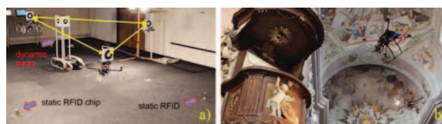
Fig. 1. Examples of practical deployment of parts of the proposed formation flying method. a) Cooperative localization of active RFID chips by a formation of relatively stabilized MAVs of a given shape. b) Documentation of hardly accessible places in historical sites by a formation of MAVs. One MAV carries a camera and its neighbors light sources with possibility to set relative angle between the camera axis and the lights, as it is required by the classical film lighting techniques, such as the three-point lighting approach [3].
