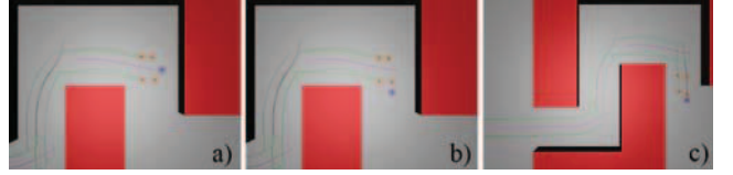
Fig. 5. Formation flying in a narrow corridor, which requires sudden changes of formation velocity to be able to fly around corners without collisions with obstacles and mutual collisions. MAVs are denoted by orange and the virtual leader by blue contours. a) The formation before the third migration of the virtual leader. b) Migration finished. c) Mission accomplished.
