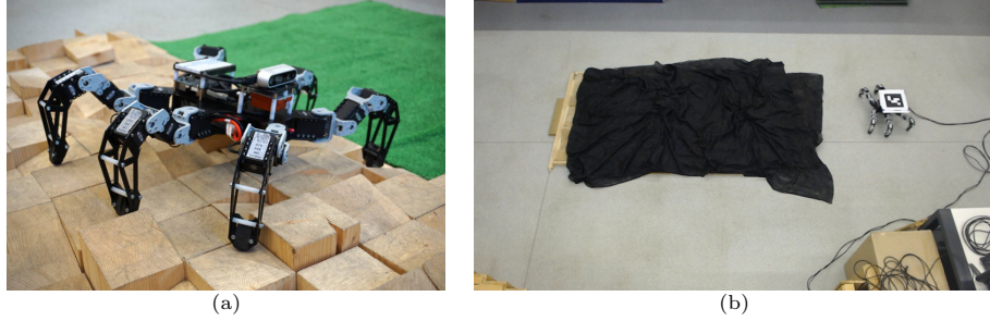
Fig. 1. (a) The utilized hexapod walking robot on the cubes terrain with turf terrain in the background; (b) and the overhead view of cubes covered with black terrain.
