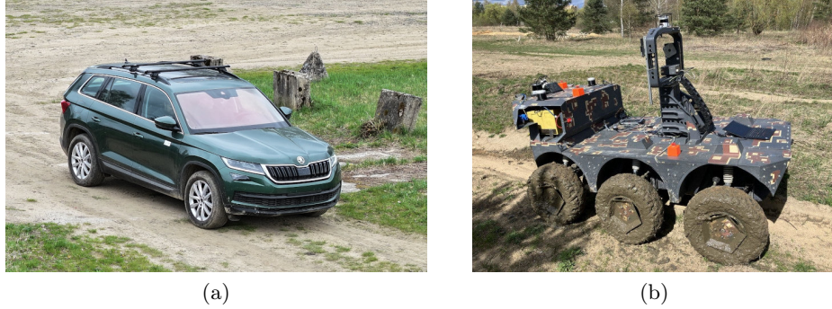
Fig. 2. (a) Škoda Kodiaq as a crewed leader vehicle; and (b) TAROS UGV used as the follower.
