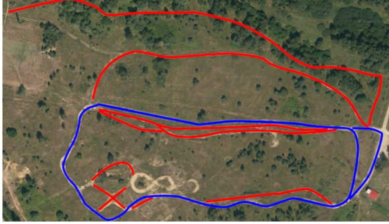
Fig. 9. An overhead view of the field testing site. The selected parts of the site include the main circuit traversed in the autonomous experiments (in blue, about 1 km long) and additional, hard-to-traverse roads that were avoided in the autonomous operation (in red) but used for data collection.
