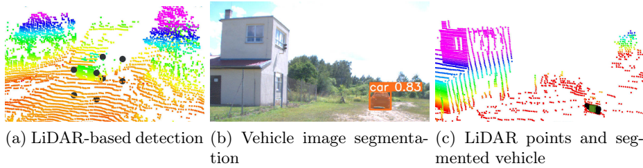
Fig. 7. (a) A LiDAR point cloud (color-coded elevation, red low, purple high) with a bounding box (in black) marking a detected vehicle. (b) Vehicle image segmentation and (c) the LiDAR points (color-coded elevation, red low, purple high) projected onto the segmented vehicle (in black, after filtering) and their centroid (green cube).
