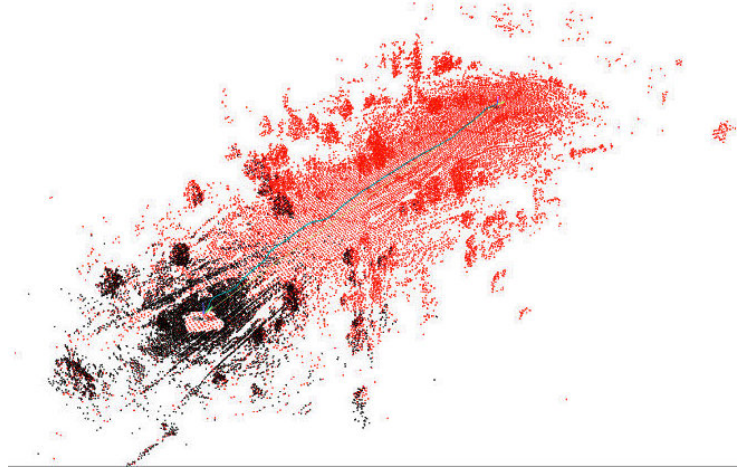
Fig. 6. Building localization map by aligning the current scan (in black) with the previously aligned scans into the point cloud map (in red). The vehicle is traveling from the top right to the bottom left.
