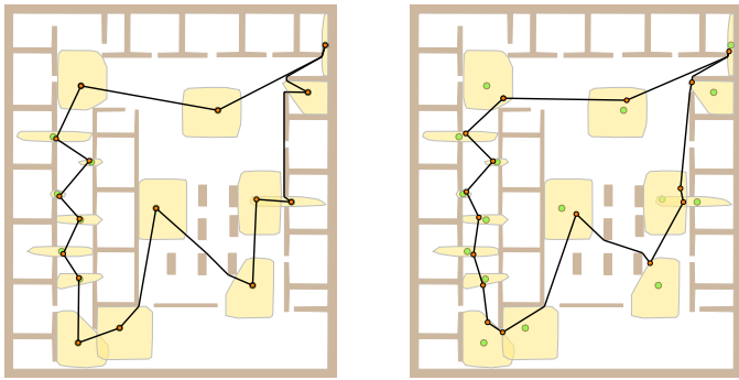
(a) a path found using termination of the adaptation if all winners are inside goals, L=78.4 m
