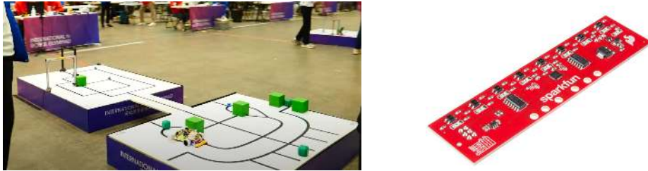
Fig. 1: A typical line follower/tracker competition (on the left) requires non-trivial programming using only one or two light sensors but can be trivially solved with six sensor bars and their associated software (on the right).
